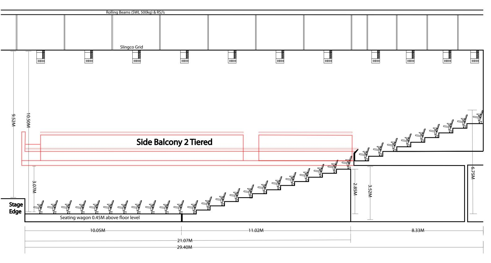
The Venue has no Fixed rigging points due to availability of rolling beams and RSJ's running full length of Auditorium. Rolling Beam SWL 500kg Riggers are able to hang heavier Drops off the RSJ's.
